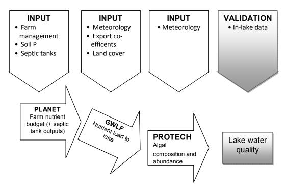
Fig. 1. Schematic of linked models and driving data used to describe the impacts of land management and septic tank use on lake water quality.
